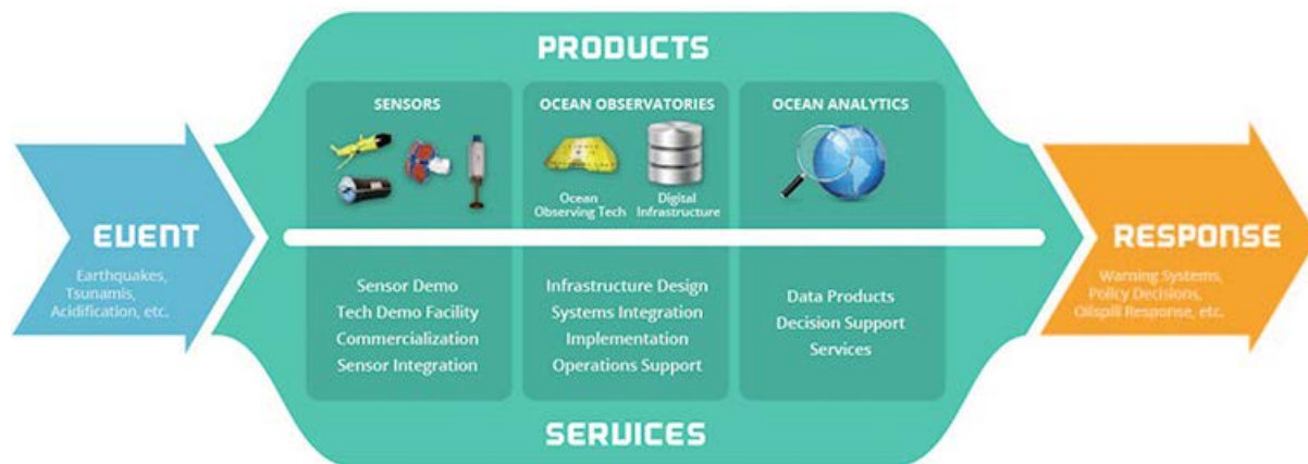
Figure 7. Smart Ocean Systems™ schematic showing the data flow elements for delivering a response (e.g. alert) to an event (e.g. tsunami).
