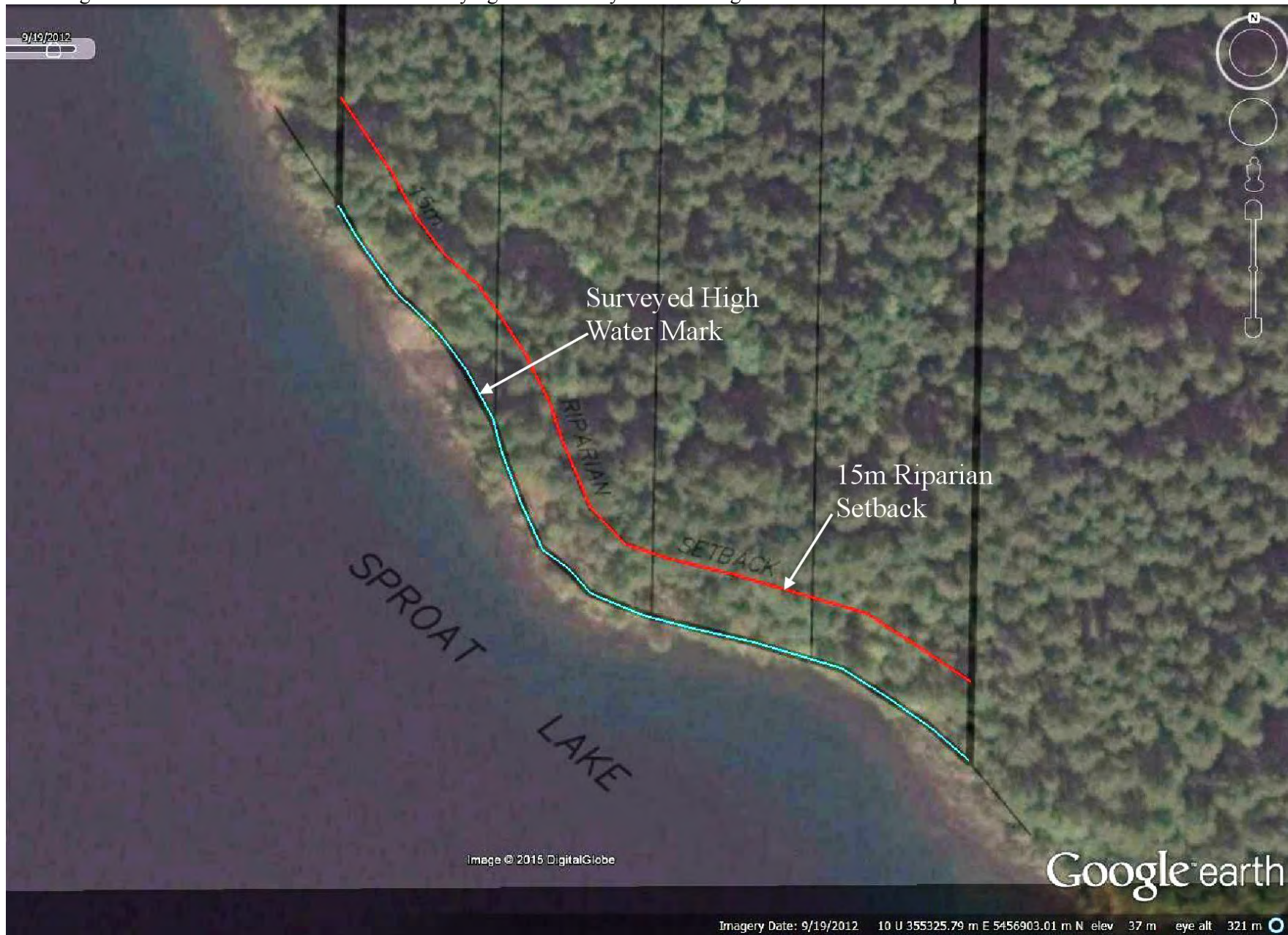
Figure 2. Part of Sims Associates Land Surveying Ltd.'s Survey Plan with high water mark and 15m riparian setbacks
