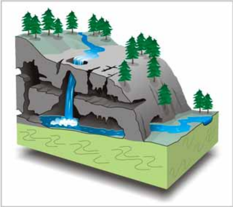
Simplified diagram of karst showing how karst functions with water entering into openings on the surface, subterranean flow, and discharge from springs (image accessed 15 Feb 2011 at www.arbucklekarst.org ).
